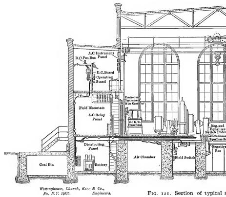
FIG. 121. Section of typical s
